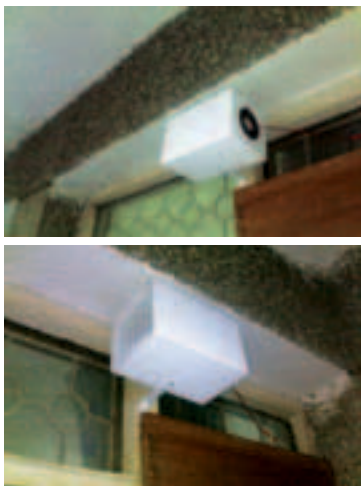
Figure 2.1a Temperature humidity logger assembly for monitoring ambient conditions
