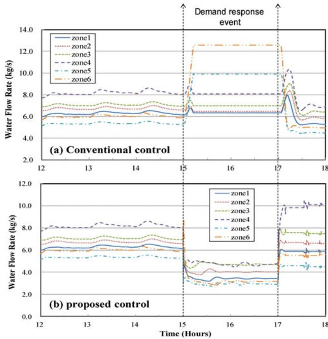
Fig. 11. Water flow profiles of zones in DR tests using conventional control strategy and proposed strategy.
