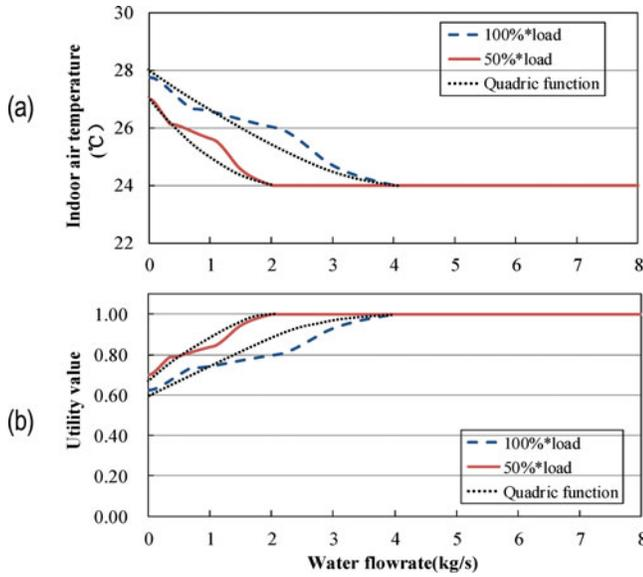
Fig. 4. Utility value versus chilled water flow rate.
