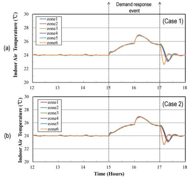
**Fig. 9.** Indoor temperature profiles of two case studies using different values of  $a$ .
