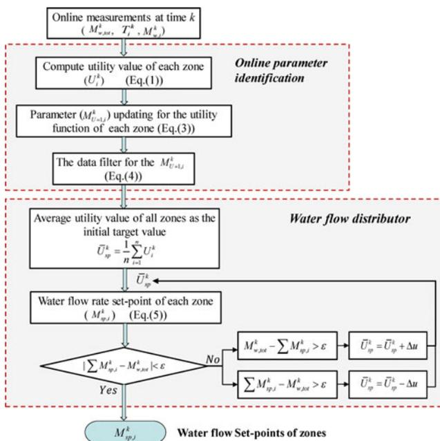
Fig. 6. Flow chart for online water flow set-point reset scheme.
