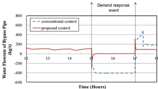
Fig. 12. Water flow rates in bypass line profiles in DR tests using conventional control strategy and proposed strategy.
