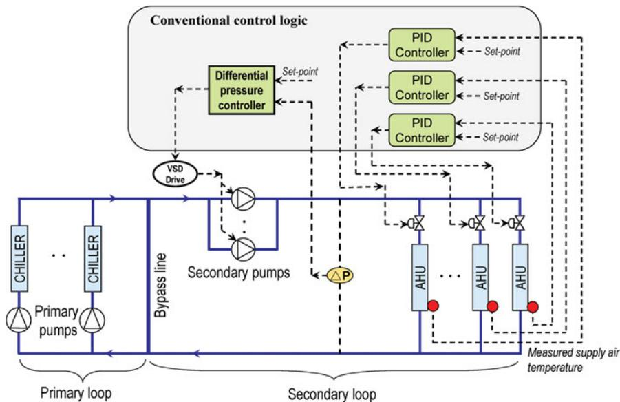
Fig. 1. Outline of a typical chilled water system control strategy used today.
