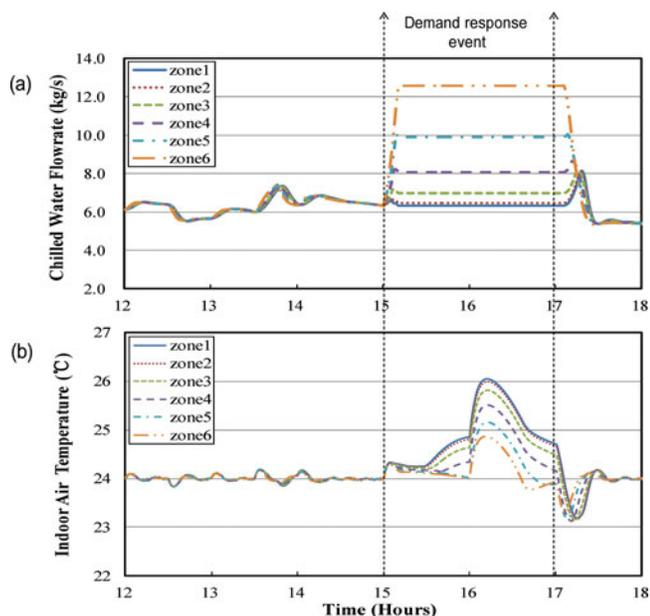
Fig. 2. Water distribution and indoor air temperature profiles of a DR test using conventional control strategy.
