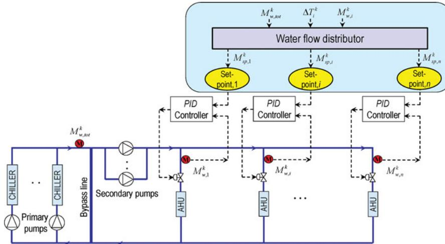
Fig. 5. Proposed chilled water flow control strategy.
