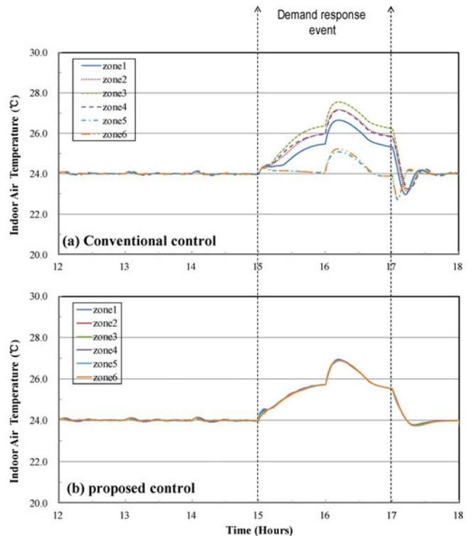
**Fig. 10.** Indoor air temperature profiles of zones in DR tests using conventional control strategy and proposed strategy.
