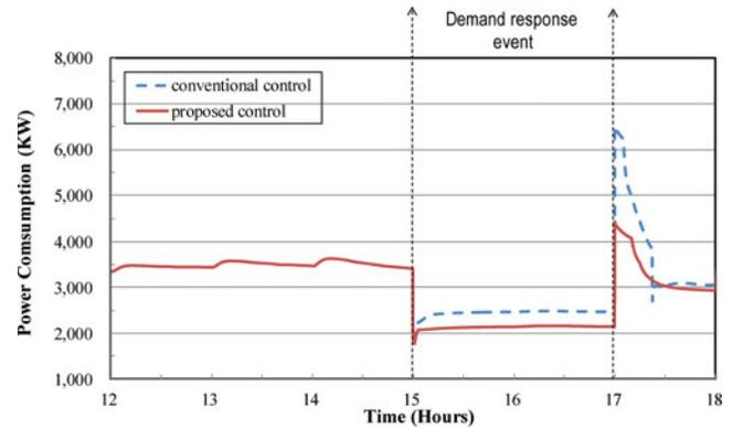
Fig. 13. Power consumptions of chillers and chilled water pumps in DR tests using conventional control strategy and proposed strategy.
