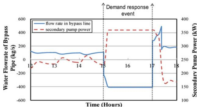
Fig. 3. Water flow rate in bypass line and secondary pump power of a DR test using conventional control strategy.
