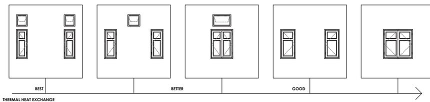
For the same ratio of area of openings to floor area of a room, the thermal heat exchange increases as the number of openings increases on the wall.<sup>29</sup> It is thus recommended to have operable ventilators to aid better ventilation.
