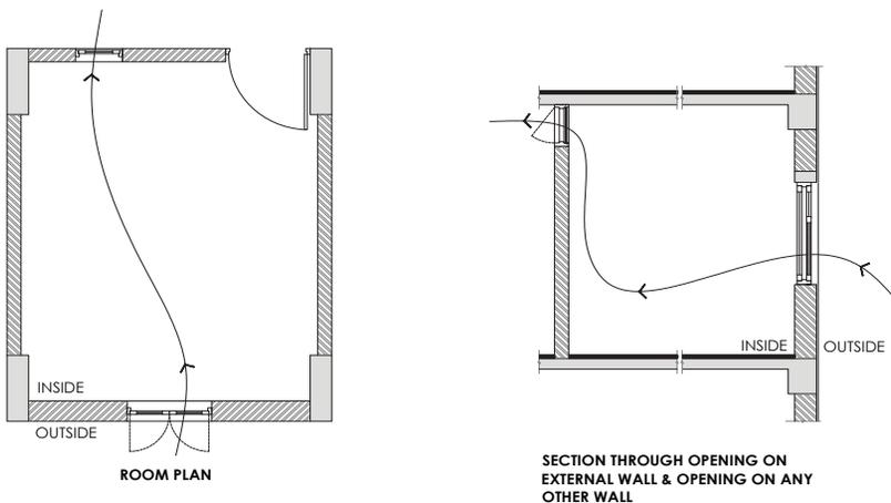
**Figure 11** Openings on external wall and internal wall for cross ventilation (Guideline)
