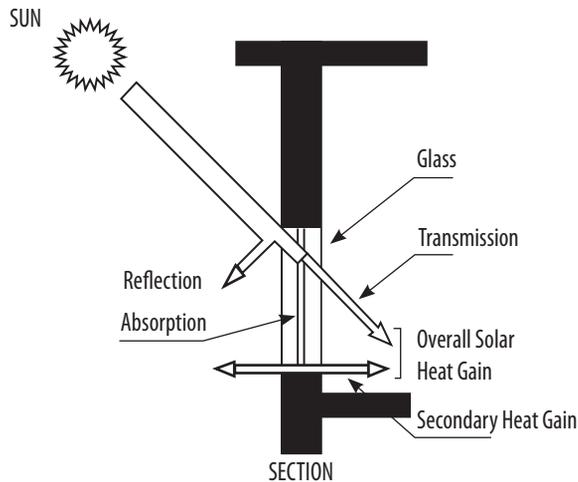
**FIGURE 4** Solar heat gain through a non-opaque component
