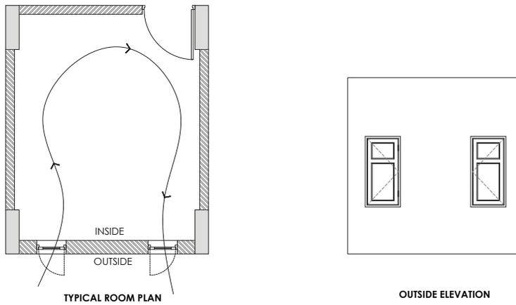
**Figure 12** Two windows on single external wall (Guideline)
