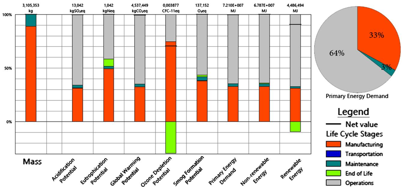
Fig. 9. Environmental impacts of the building based on a standard design.
