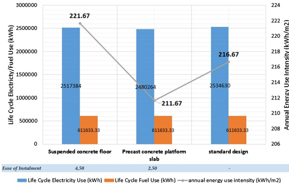
Fig. 6. Comparison of the floor and ceiling components applied in the case study.
