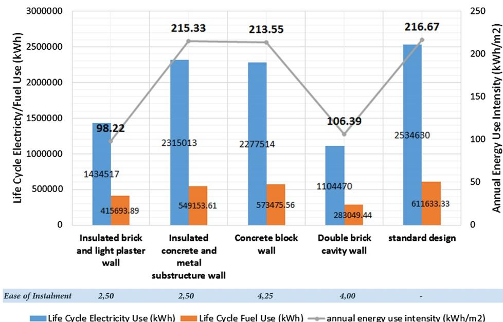
Fig. 5. Comparison of the exterior wall components applied in the case study.
