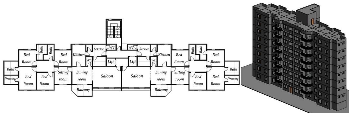
Fig. 4. 2D and 3D plan of the multi-story residential building used as a case study.
