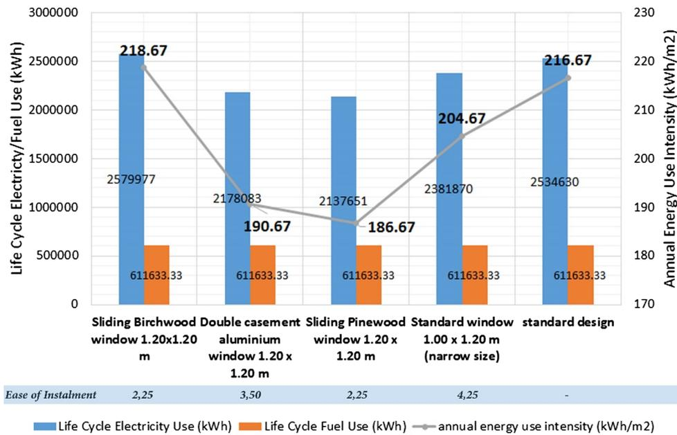
Fig. 7. Comparison of the window components applied in the case study.
