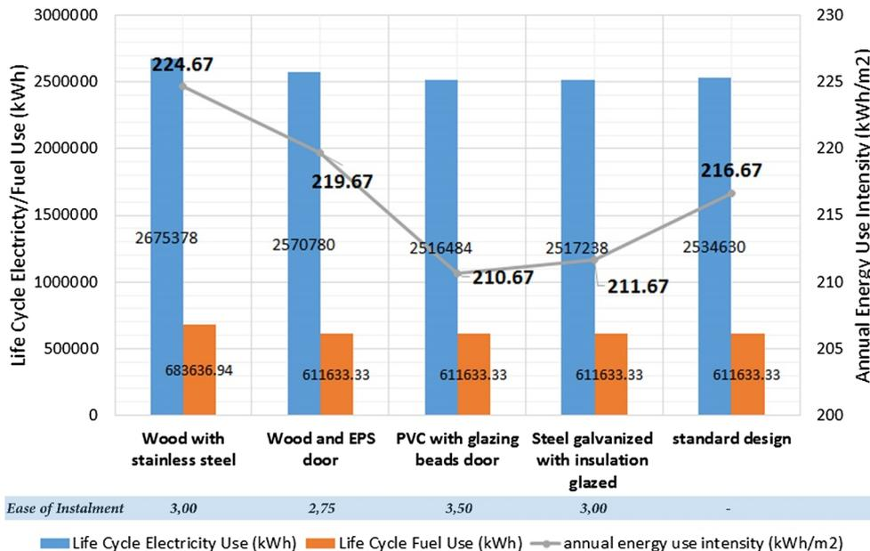
Fig. 8. Comparison of the door components applied in the case study.
